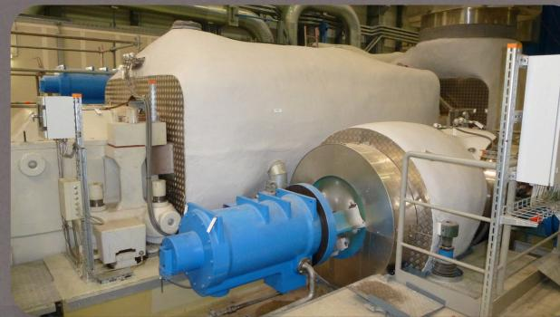
If a protective, durable coating is required, LIMPET BD6, a factory premixed, cement-based, self-hardening finishing coat, can be used on calcium silicate and all types of mineral wool-based thermal insulation.
